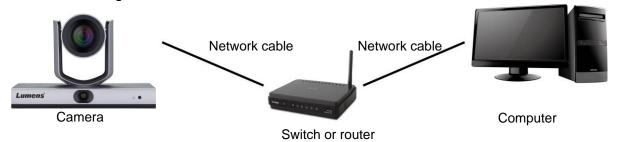
2. To connect directly through network cable, the IP address of the computer should be changed so that it is on the same network segment as the camera E.g.: The factory-preset default IP address of VC-TR1 is 192.168.100.100. The computer IP address must be set with the same network segment, such as 192.168.100.101, so that the computer can be connected correctly with the camera
